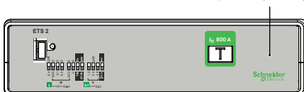
LSI Protection - Electronic Trip Unit (ETS 2)
